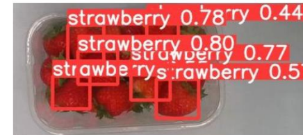
Fig 38 – Sample screen grab of the results of the vision algorithm : strawberry identification
